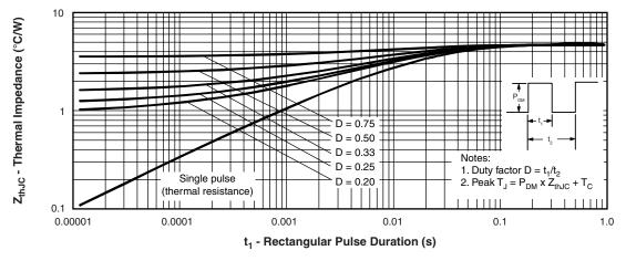
Fig. 4 - Maximum Thermal Impedance Z<sub>thJC</sub> Characteristics (Per Leg)
